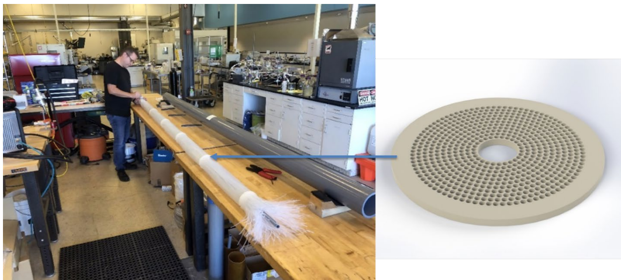
Figure 5: 4-Inch P-HEX Tube Bundle Assembly With Spacers
