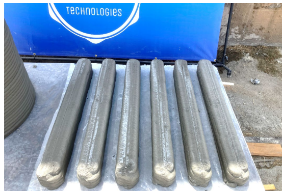
Figure 25. Printed Beam Samples for Quality Testing
