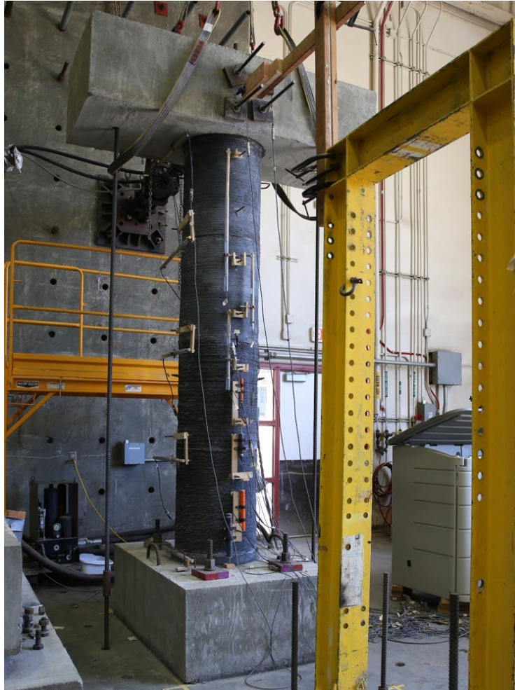
Figure 8. 3D-printed Concrete Tower and Test Setup
