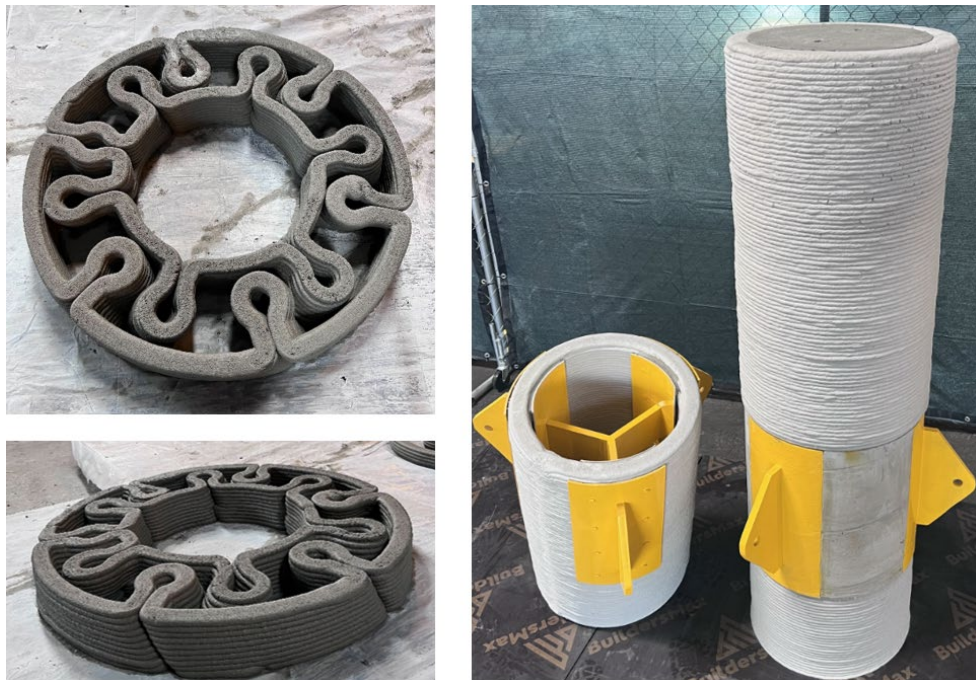
Figure 27. 3D-printed Concrete Anchor Prototypes
