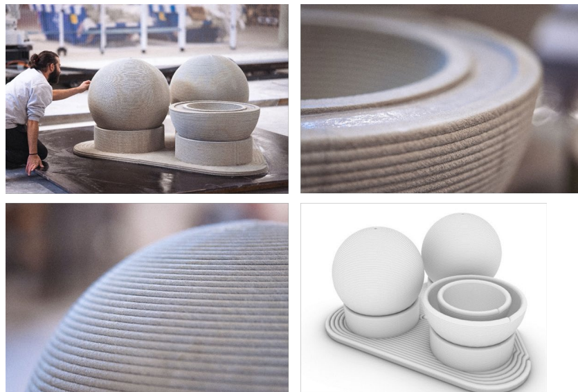
Figure 28. Photographs of the Prototype 3D-printed Concrete Underwater Energy Storage Spheres
