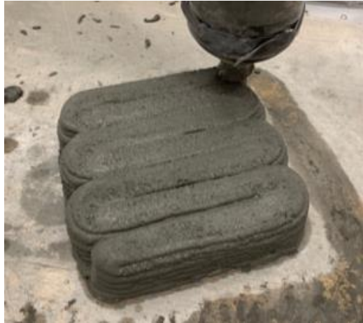
Figure 16. Printed Sample of 78-MPa Recycled 3D-printable Concrete
