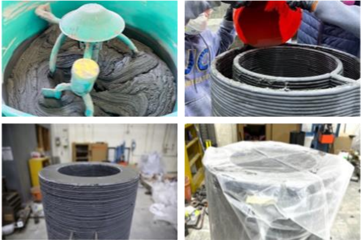
Figure 9. The Mixing, Casting, and Curing Process of the Tower Segment
