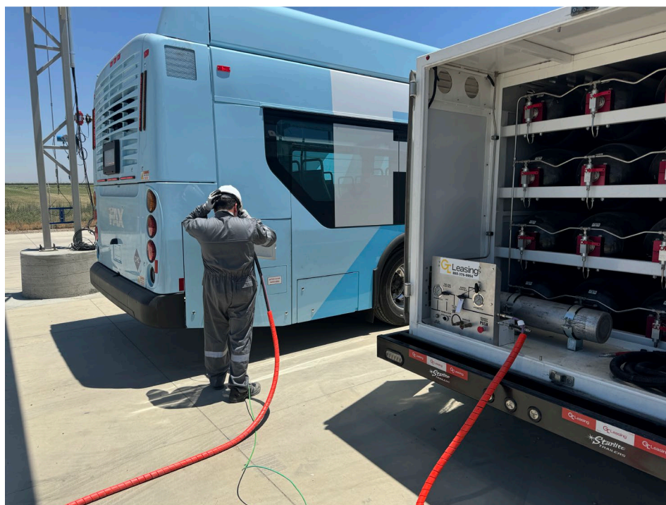
A FAX bus is being refueled using the GTL Leasing gaseous hydrogen trailer.
