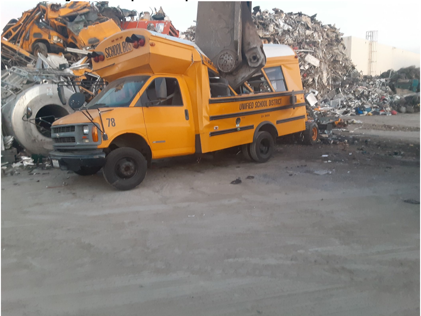
Figure 2: Example of Acceptable Method to Dismantle Vehicle
