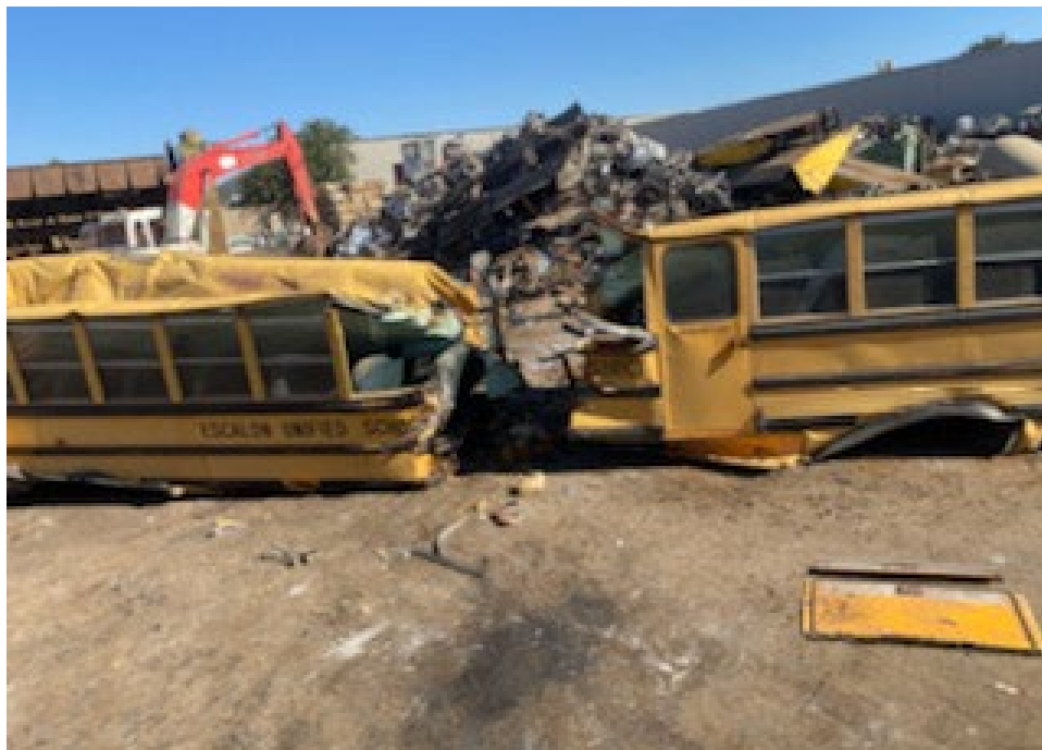
Figure 2: Example of Acceptable Method to Dismantle Vehicle Chassis
