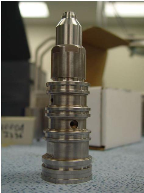
**A: Assembled injector (less feed orifices, screens, o-rings, and actuators)**
