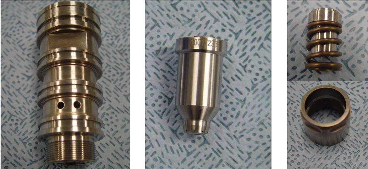
**Figure 11: Photos of J236 injector components and assembly as received from the supplier**
