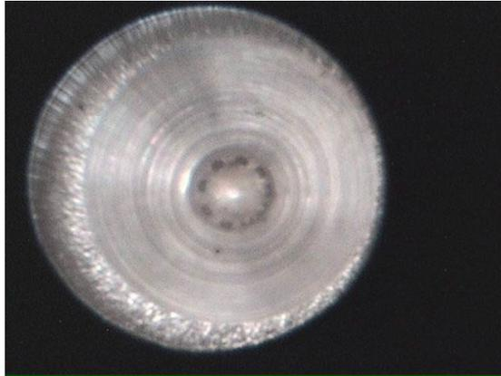
**Figure 17: Needle seating surface after engine test (red marking was added after disassembly to aid alignment inspection)**
