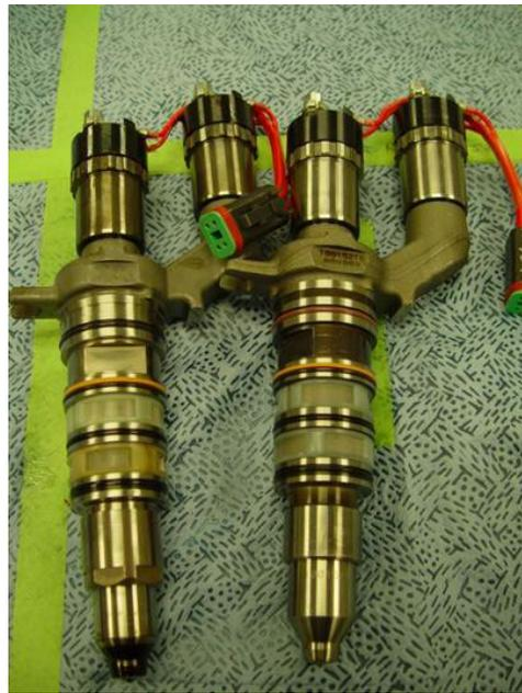
**B: Comparison of new fully assembled J236 (right) with stock J36 (left)**
