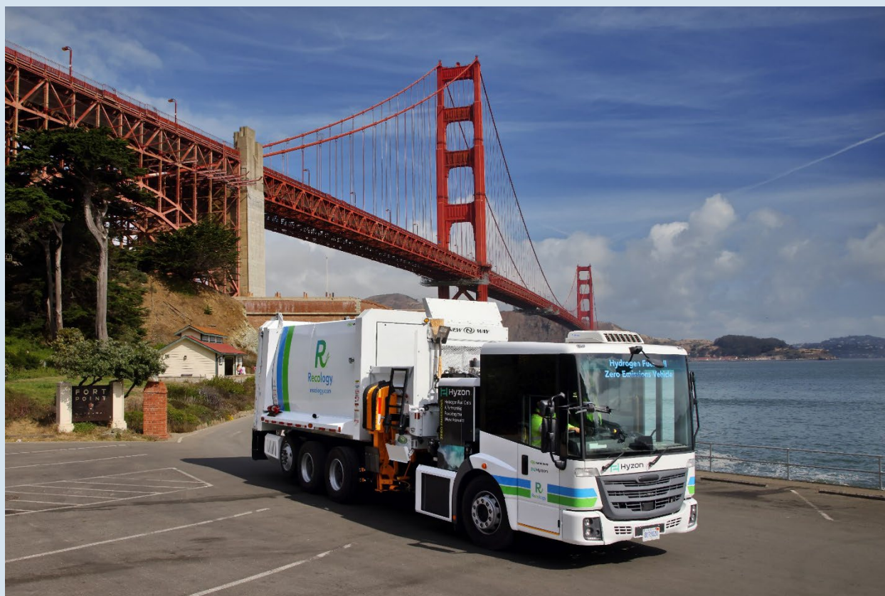
FIGURE 17: RECOLOGY HYDROGEN FUEL CELL REFUSE COLLECTION TRUCK
