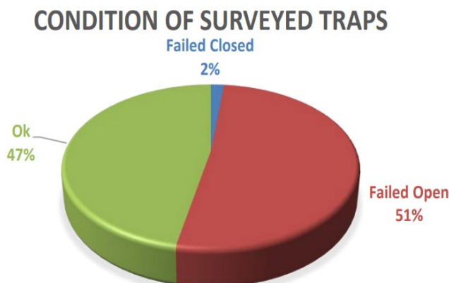
Figure 6: Condition of Old Steam Traps
