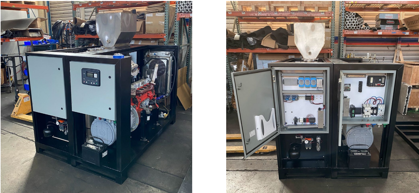
Figure 10: Side-by-side Gas-Making and Power Gen Automation Enclosures
