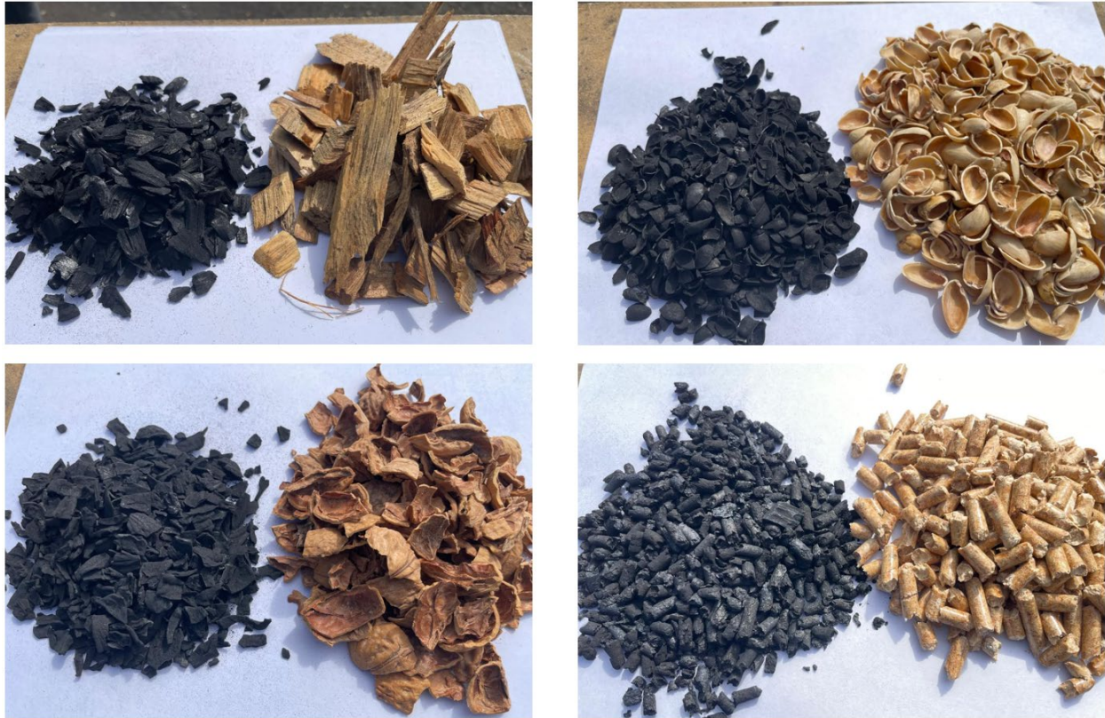
Figure 13: Biochar and Feedstock - Wood Chips, Pistachio Shells, Wood Pellets, Walnut Shells
