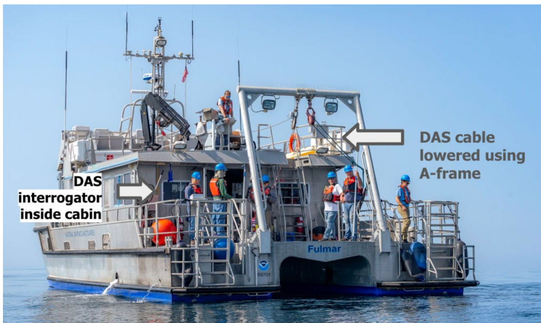
Figure 16: Research Vessel in Monterey Bay With DAS Interrogator Housed Inside the Cabin and DAS Cable Lowered to the Water Using A-Frame
