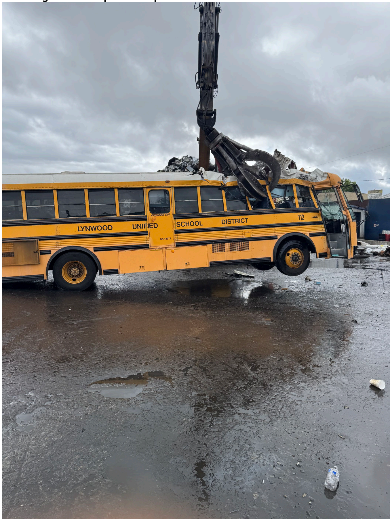
Figure 2: Example of Acceptable Method to Dismantle Vehicle Chassis
