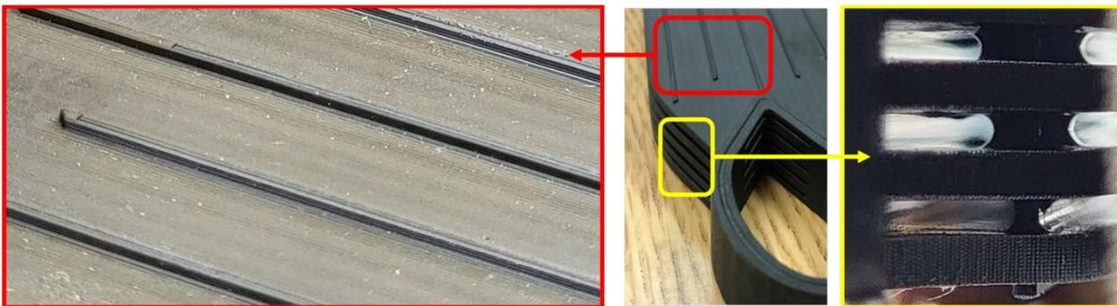
**MPHX Core Outer Wall at the end of experiments, inset picture shows a few air channels with no visible sign of failure.**
