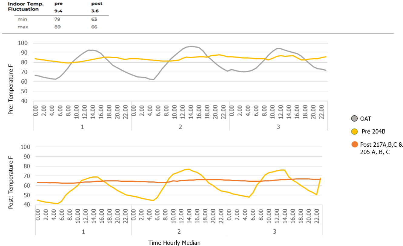
Figure 14: Corona Del Rey: Apartment Indoor Air Temperatures Relative to Outdoor Air Temperatures, Pre-and Post-retrofit
