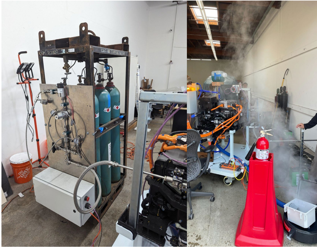
Figure 3: Fuel Cell Test Stand Hydrogen Delivery System and Commissioning Exhaust
