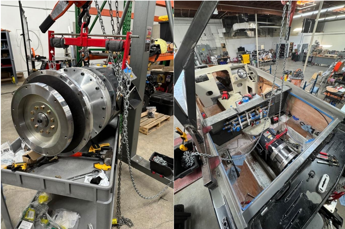
Figure 7: Vessel Electric Motor and Drive Train Coupling
