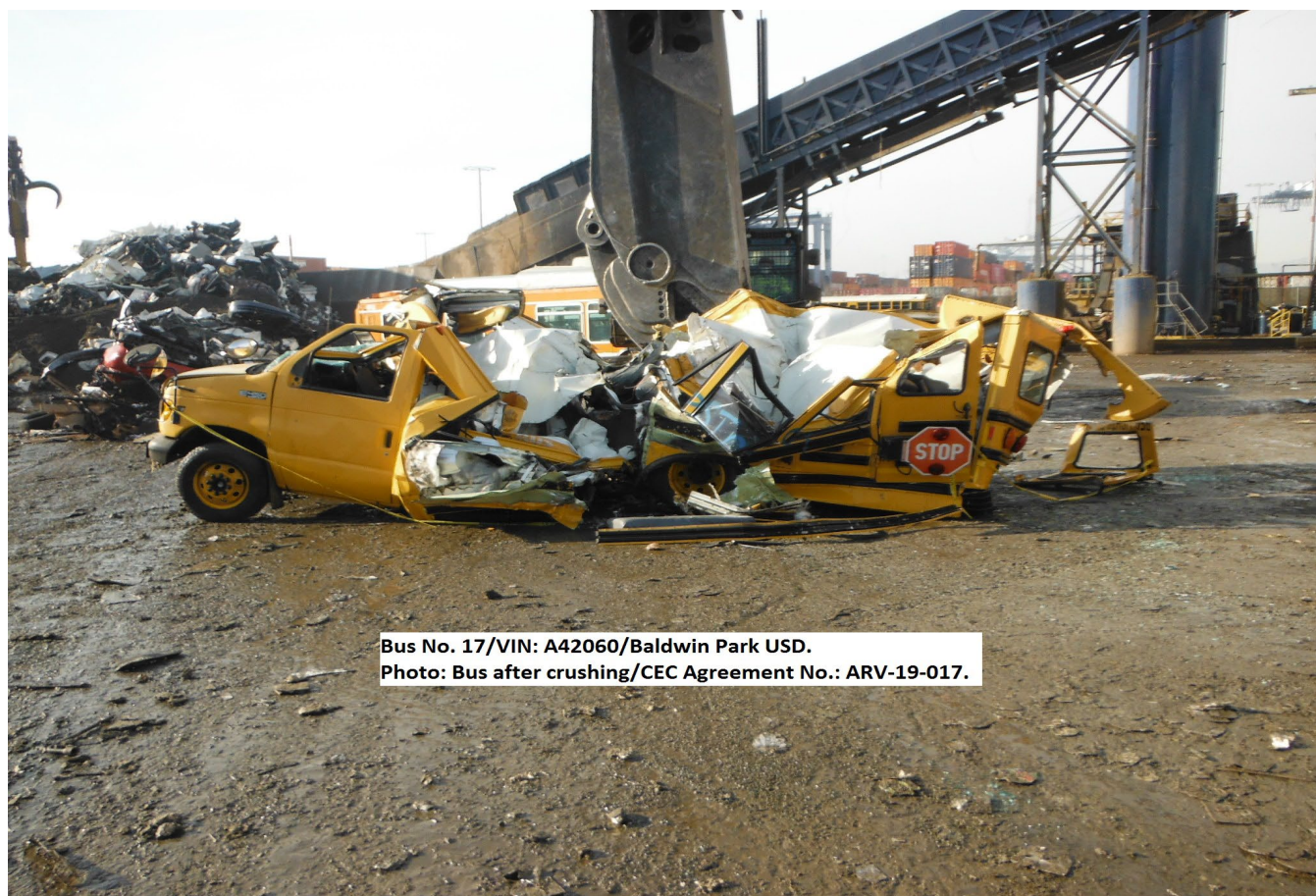
Figure 2: Example of Acceptable Method to Dismantle Vehicle Chassis
