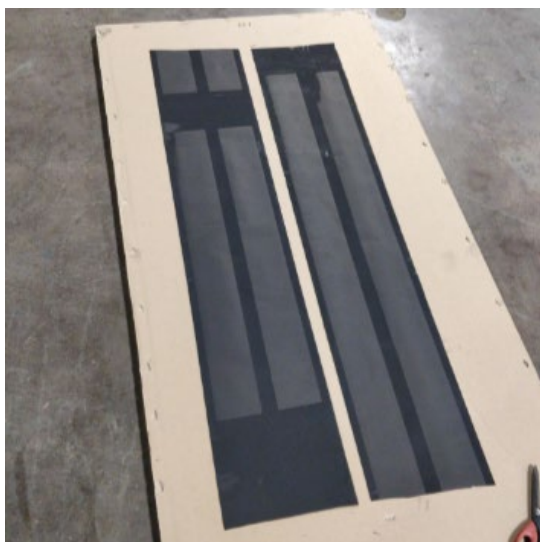
Figure 12: Initial Production Runs of Positive Electrode at Contract Manufacturers, Showing Poor Quality of the Coated Positive Electrode Material
