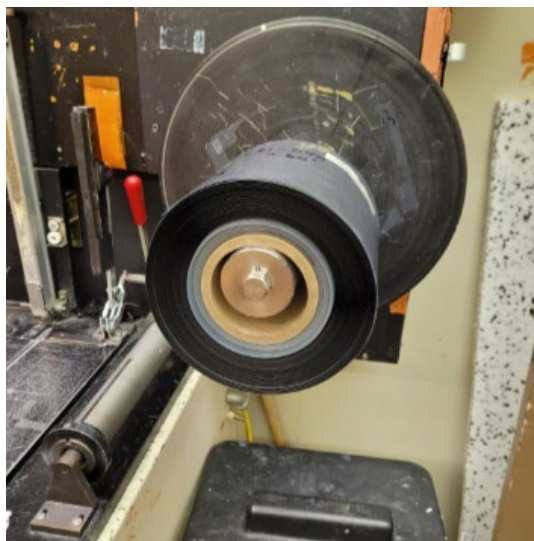
Figure 13: Slot-Die Coating Head Coating Zn-ion Cathode (left): ~40 m Roll of Dried Zn-ion Cathode (right)
