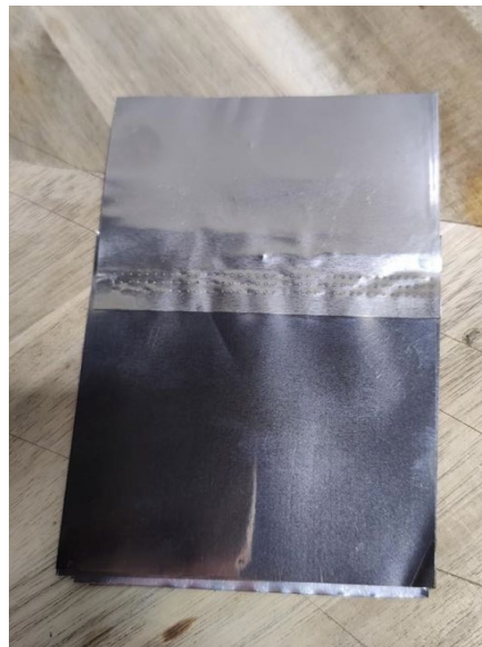
Figure 22: Example of Laser-Welding the Electrode Tabs/Terminal of a Zn-Ion Cell
