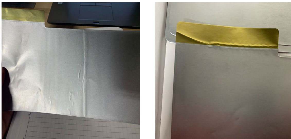
Figure 20: Examples of Defects Identified in Negative Electrode Production, Folds and Bends (left) and Creased Tab (right)
