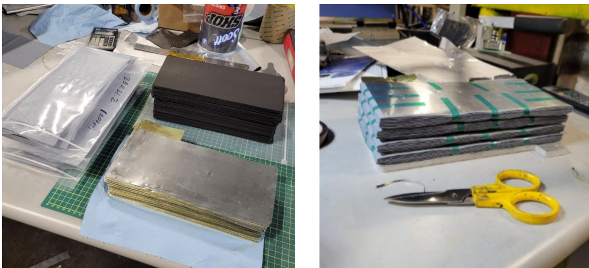
Figure 6: 20-Ah Zn-ion Pouch Cell Subcomponents Before Cell Stacking (left); 20-Ah Zn-Ion Cell Stacks (right)
