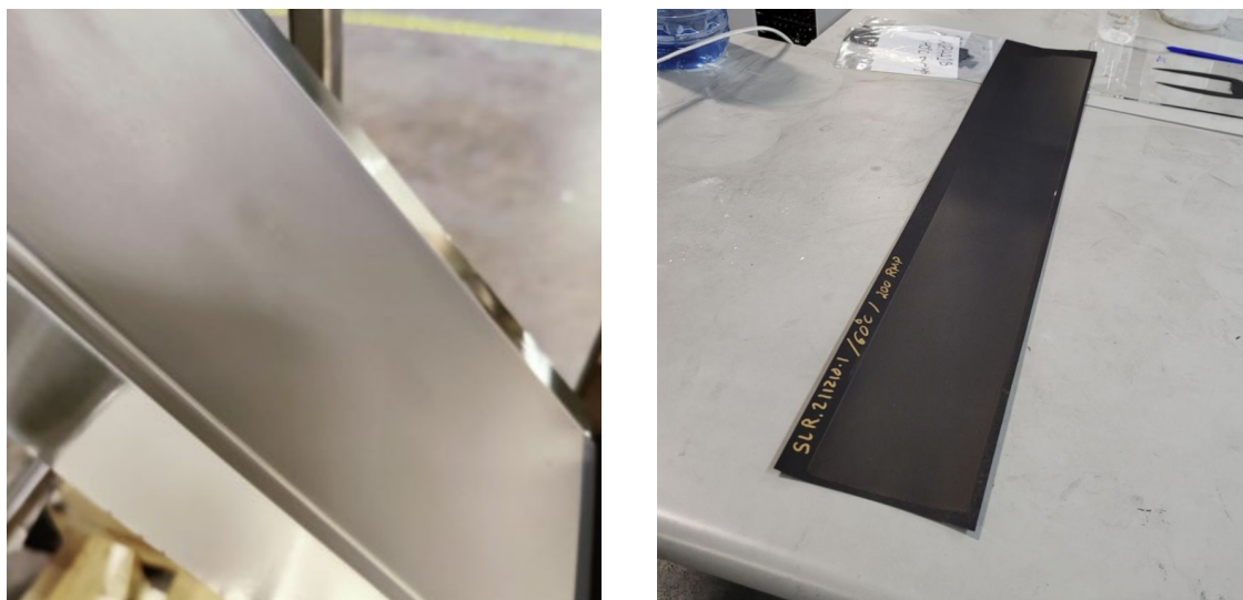
Figure 11: Dried Positive Electrode Following In-House Roll-to-Roll Process Development
