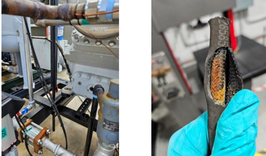
Figure 16: Bulging of Ammonia Oil Return Hose and Rust within Hose Jacket
