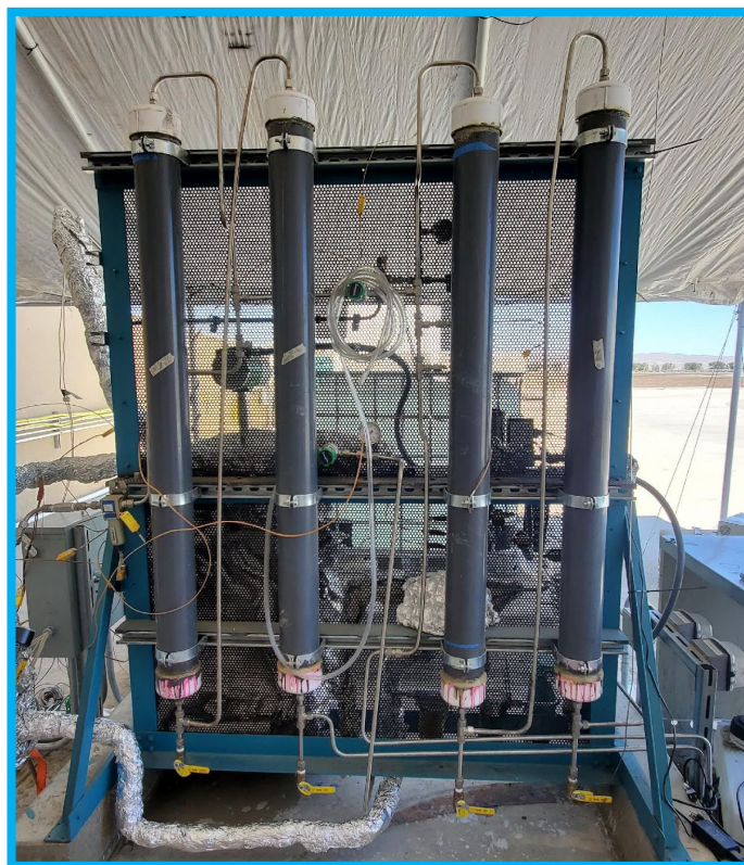
Figure 12: USC Catalytic Reformer deployed at the project site
