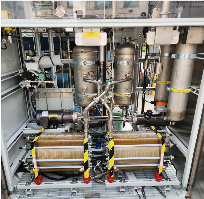
Figure 8: Alkaline Electrolyzer and High-Pressure Hydrogen Storage
