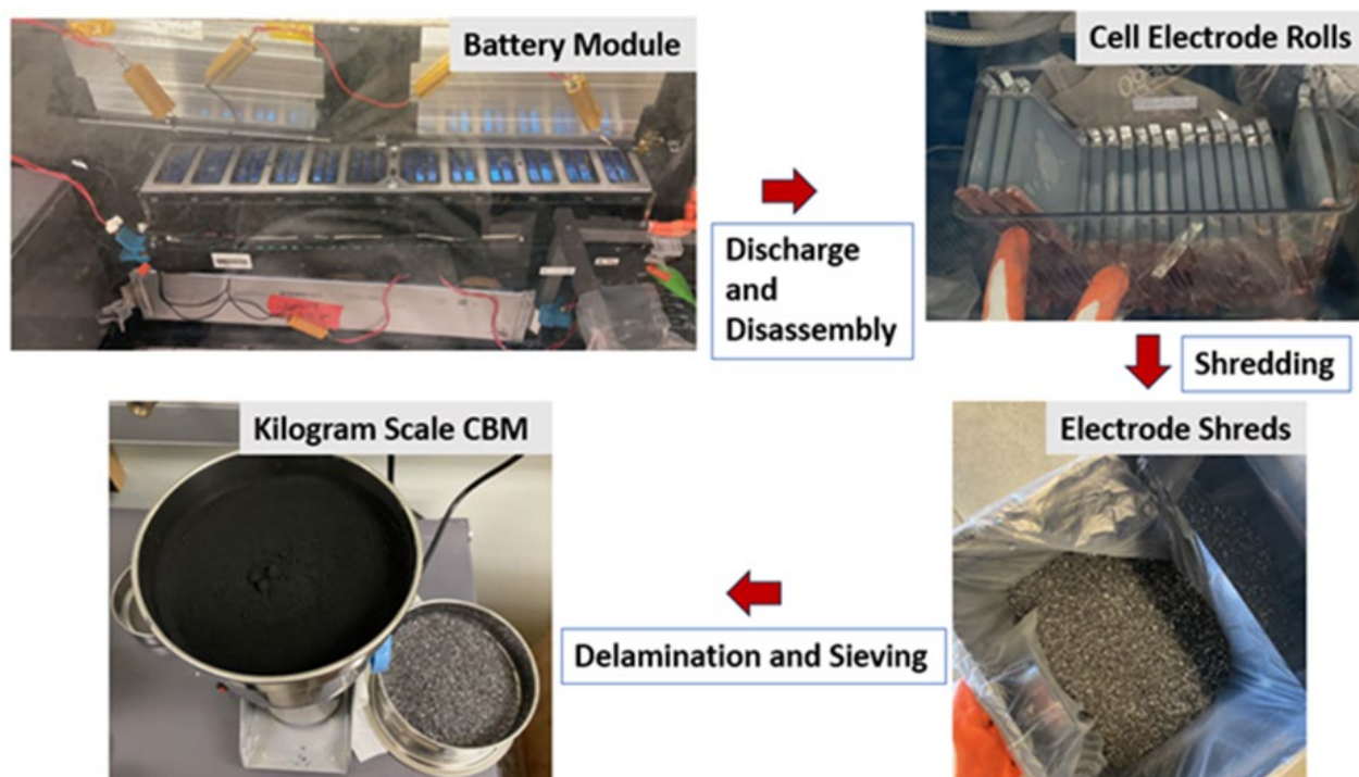
Figure 15: Preprocessing Schematic to Obtain CBM From the Battery Modules Obtained From Spent EV Packs Received From Vendor B
