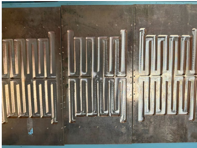
Figure 9: Water Channels Machined on Back Side of New Heat Sink Copper Plate
