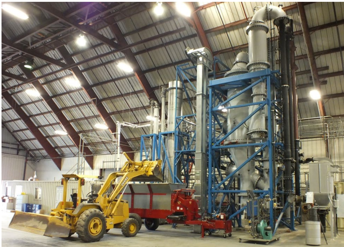
Figure 2: Pilot-Scale Gasifier at The Woodland Biomass Research Center
