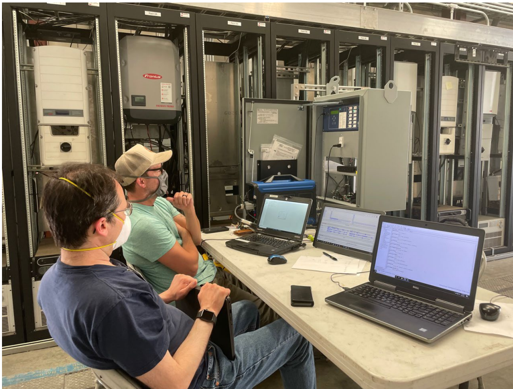
Figure 22: Bench Testing the SEL-651R Recloser Control
