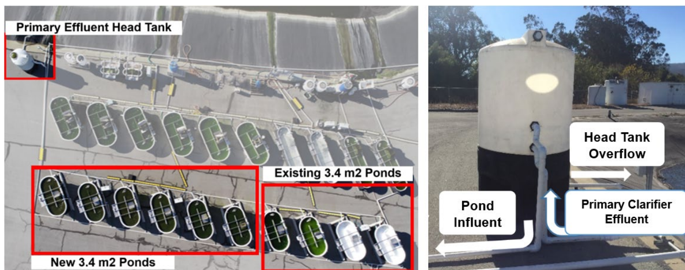
Figure 18: Pilot System Layout and Primary Effluent Head Tank Configuration at SURE! Field Station
