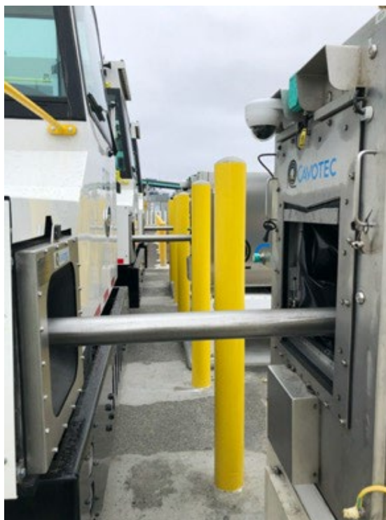
Figure 5: BYD's Zero-Emission Yard Tractors Connected to Cavotec's SPS
