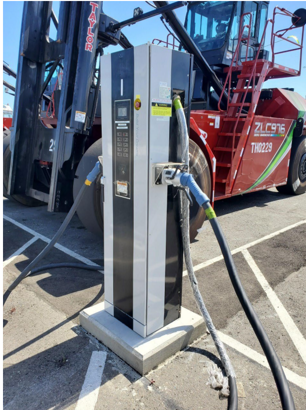
Figure 4: Taylor's Zero-Emission Top Handler and BYD's EVSE
