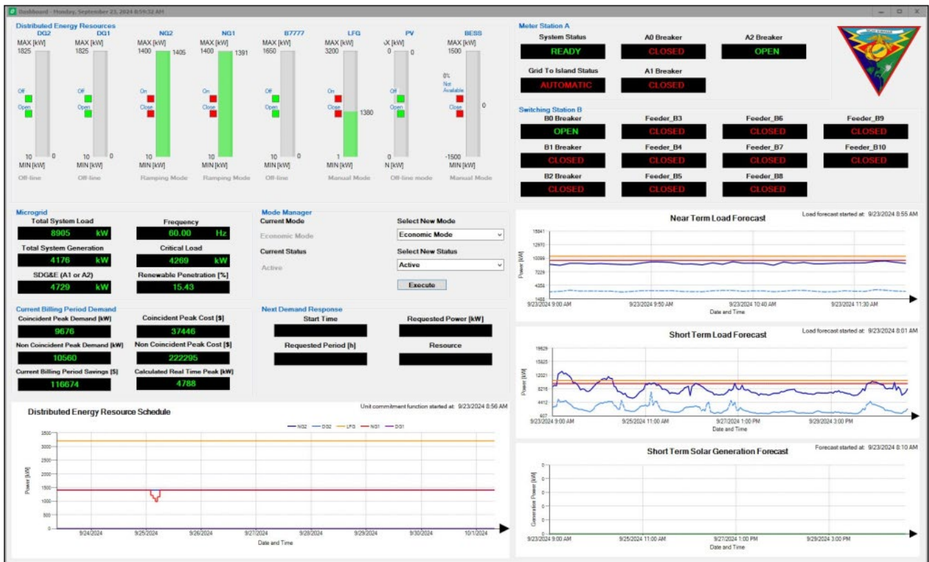
Figure 7: PCS Microgrid Monitoring and Control Screen
