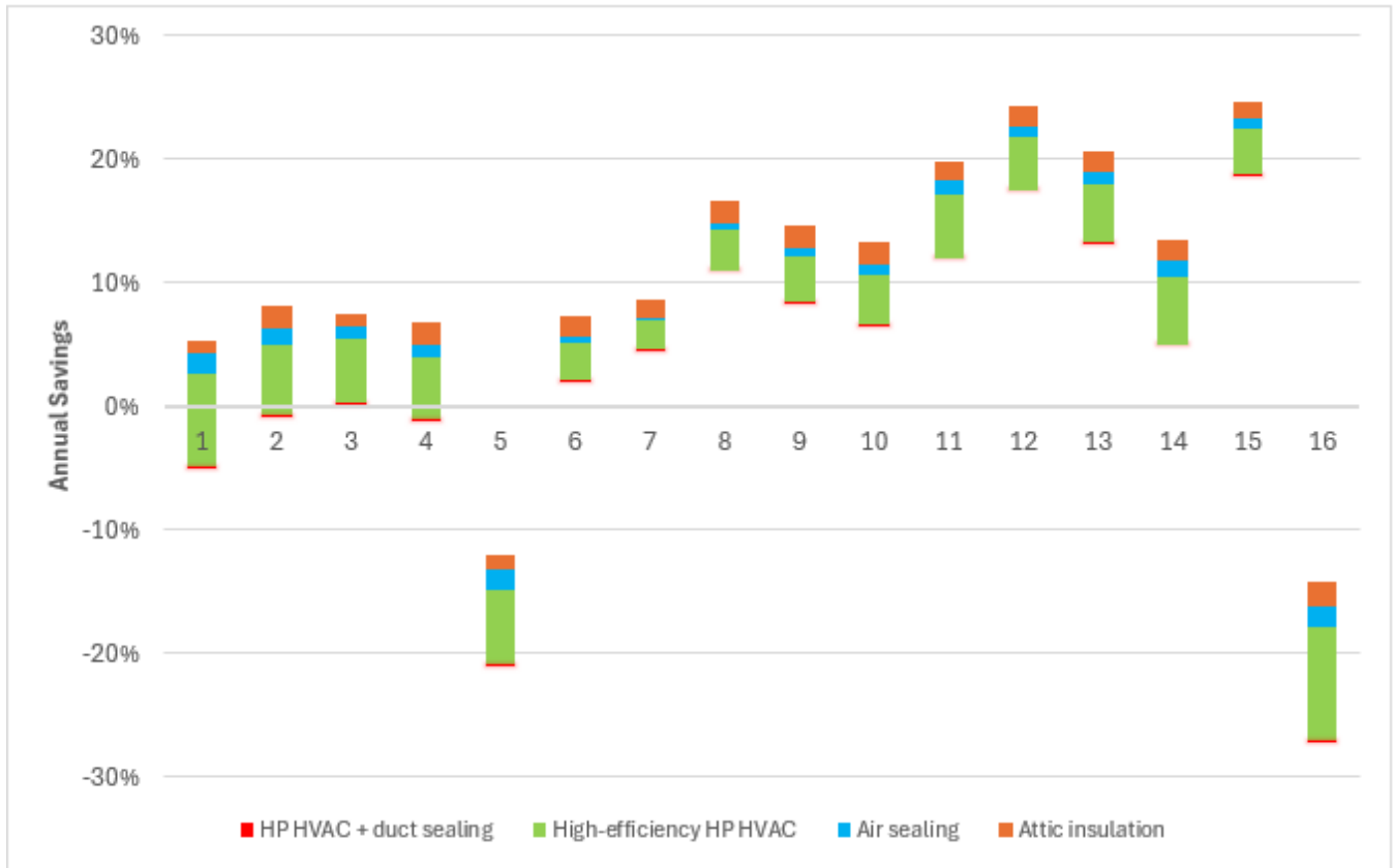
Figure B-11: Annual Bill Savings for HP HVAC With Incremental Measures by Climate Zone
