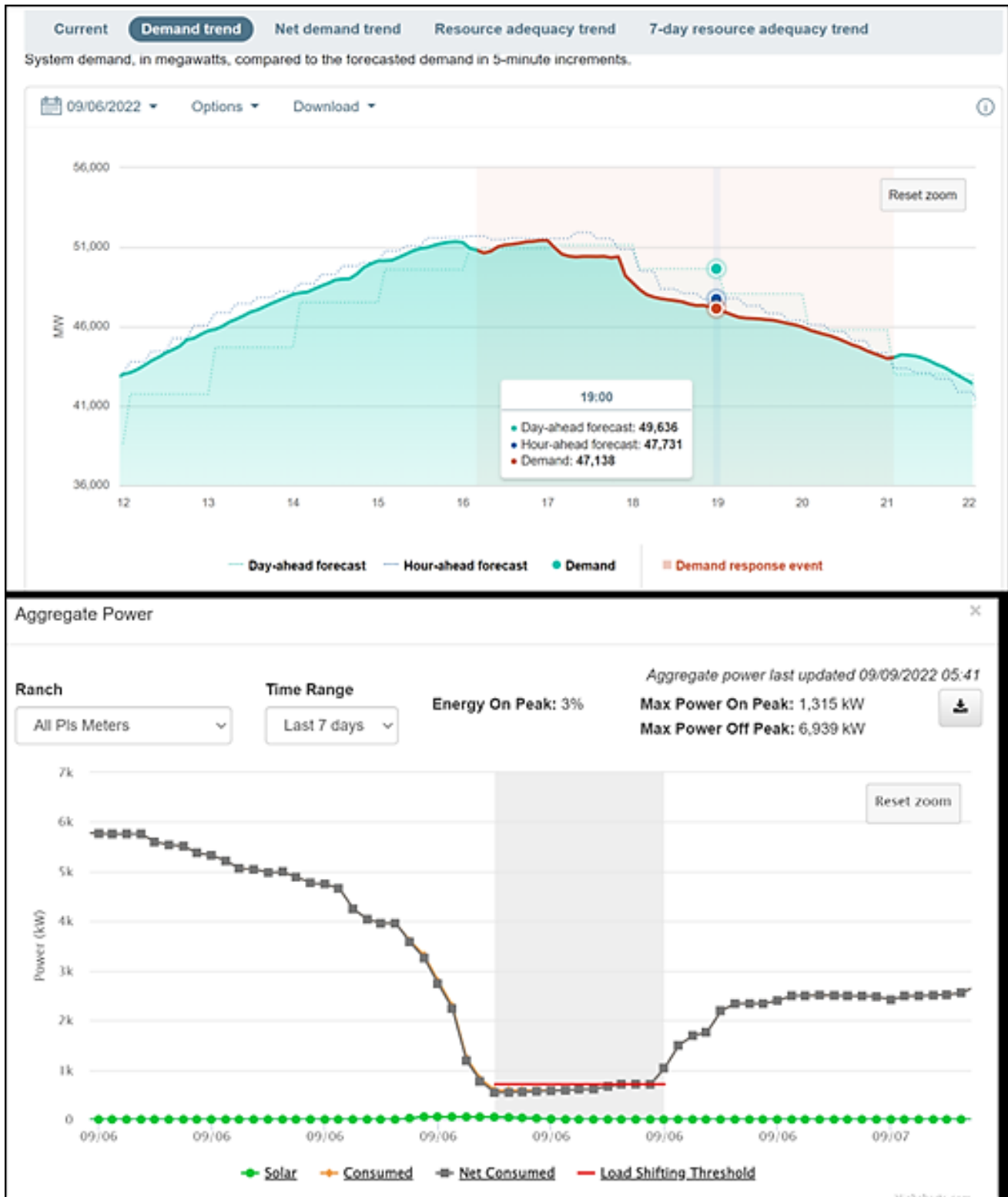
Figure 11: Total Power Load Shed Statewide (top) Versus Load Shifted by Implementation of the PLS Program (bottom) During the Emergency Event of California ISO on September 6, 2022
