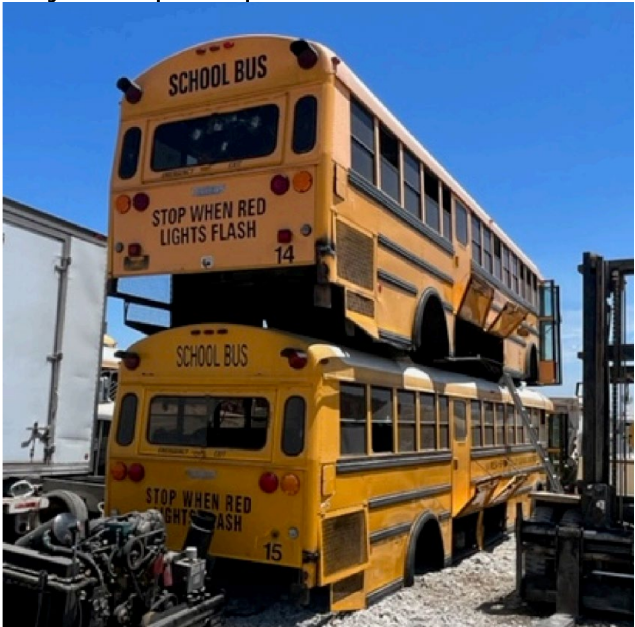
Figure 3: Example of Acceptable Method to Dismantle Vehicle Chassis
