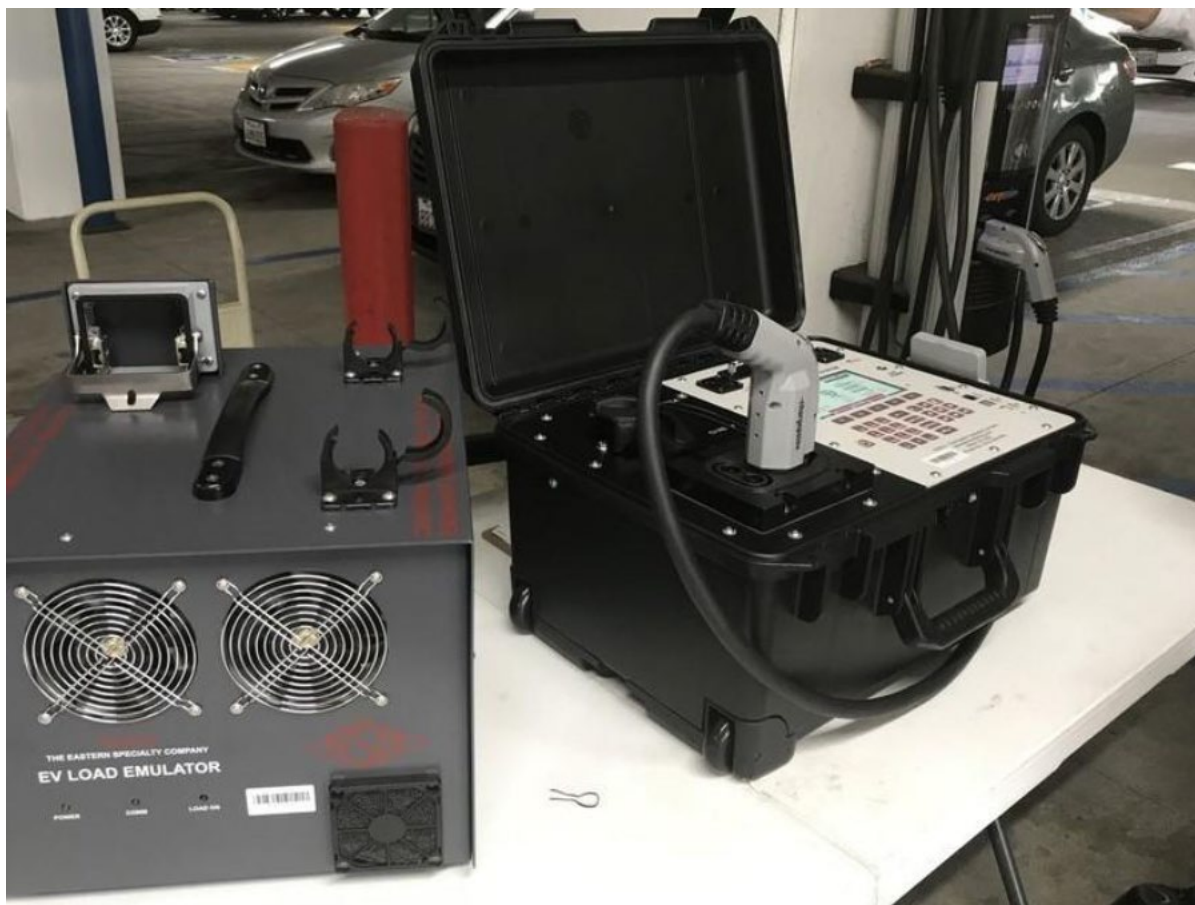
Example of Field standard and load emulator used for testing installed commercial EVFS
