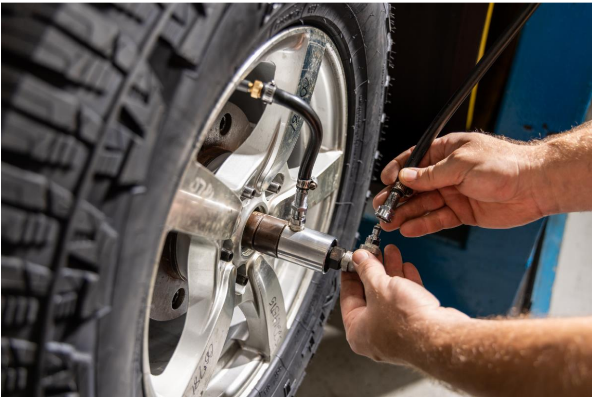
Photograph A5.2: Connecting Tire to Air Pressure
