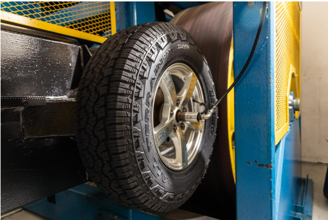
Photograph A5.6: Tire Ready for Testing
