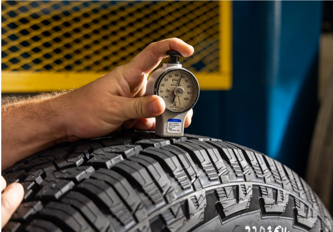
Photograph A5.3: Measuring Tread Hardness
