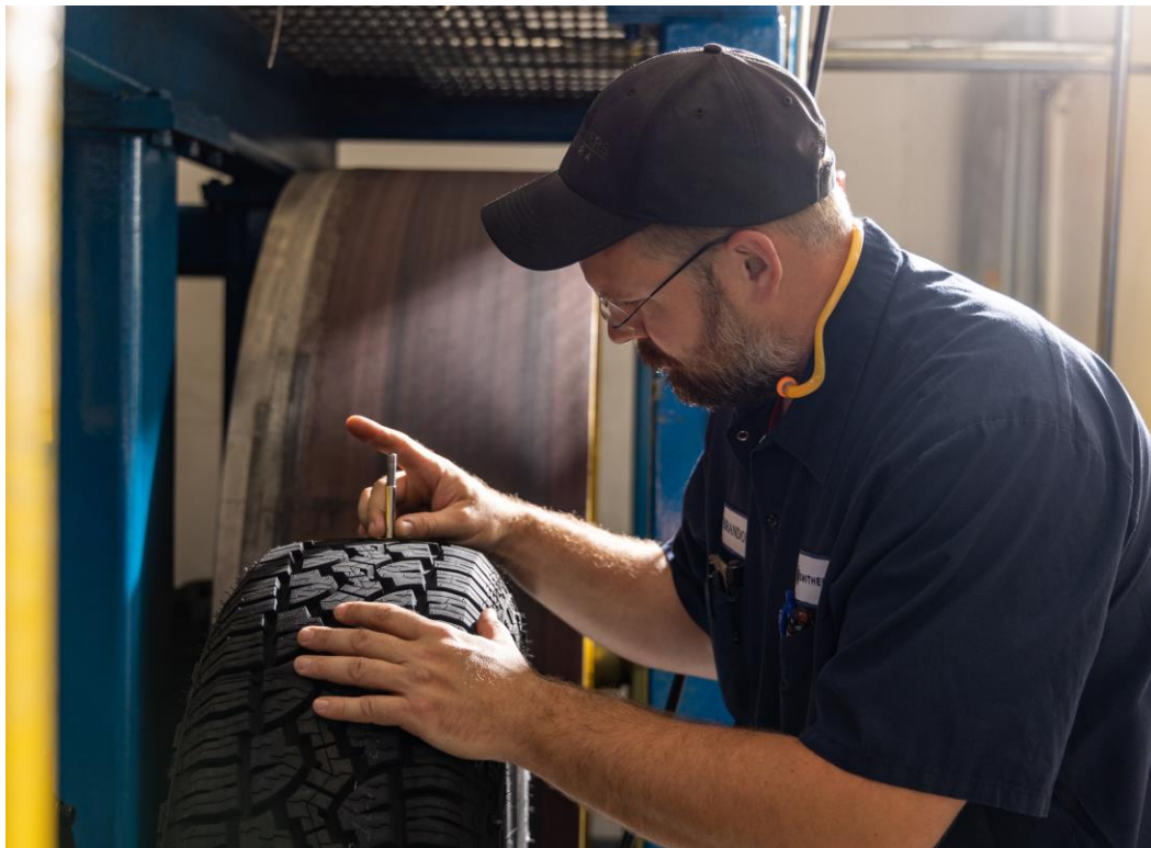
Photograph A5.4: Measuring Tread Depth
