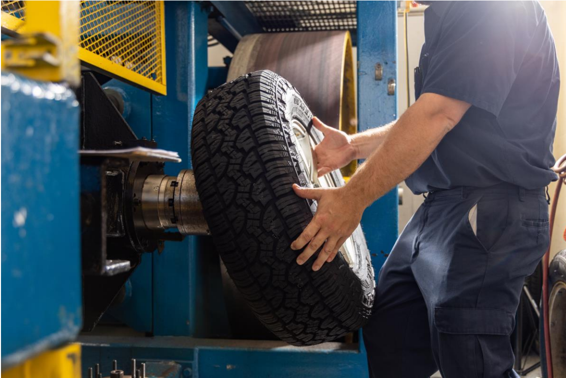
Photograph A5.1: Mounting Rolling Resistance Tire
