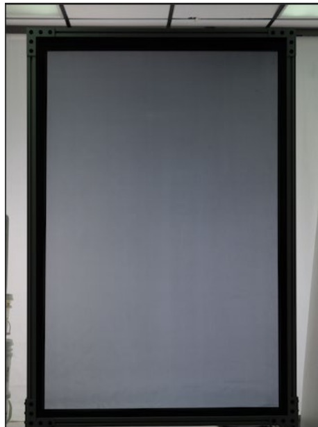
Figure 9: Single 40" x 60" Window-PV Unit with High Aesthetic Quality
