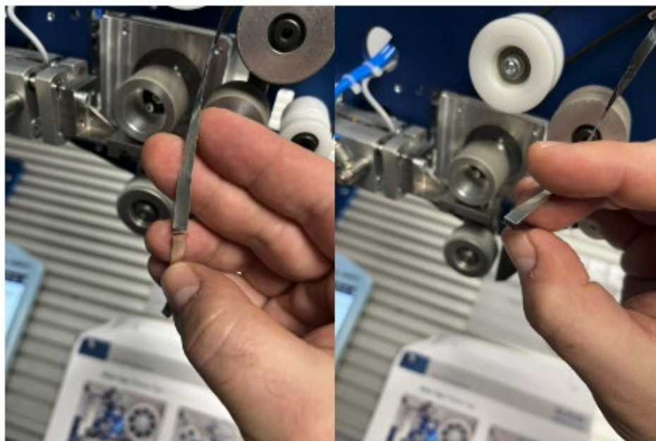
Figure 3: Bus Bar Cut Quality
