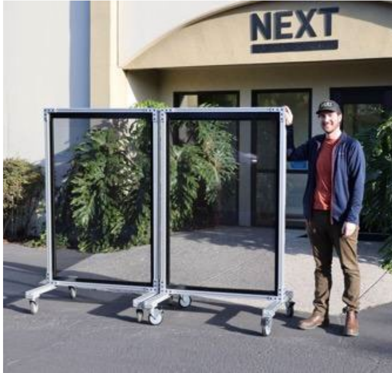
Figure 10: Two 40" x 60" Window-PV Modules for Display
