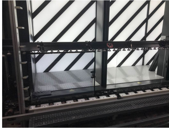
Figure 12: IGU Fabrication Process at Viracon with OPV Lite Integration
