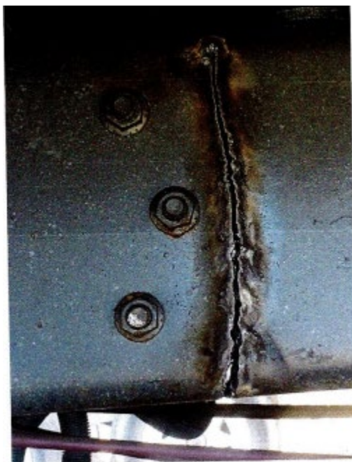
Figure 2: Chassis Rail Cut in Half
