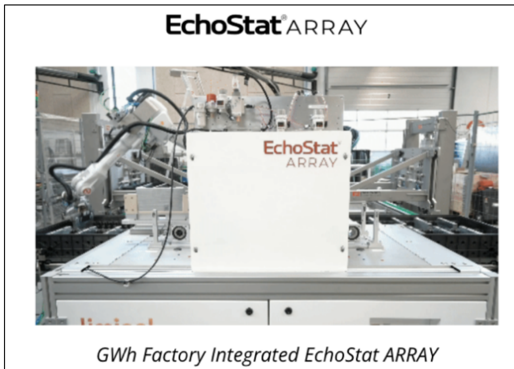
Figure 16. EchoStat ARRAY 5 System Fully Automated and Integrated In-line at NorthVolt Meeting the Line Throughput Requirements (10 parts per million) and Detecting Six Defect Types with >95 Percent Accuracy.
