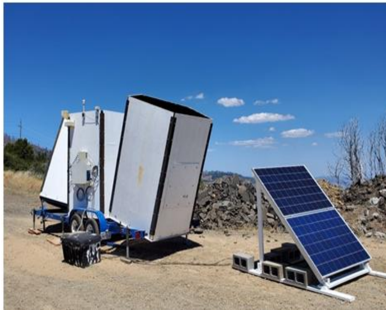
Photograph of the ACS Model 2000 Sodar system used at the upper-air monitoring site near Cobb Mountain, California
