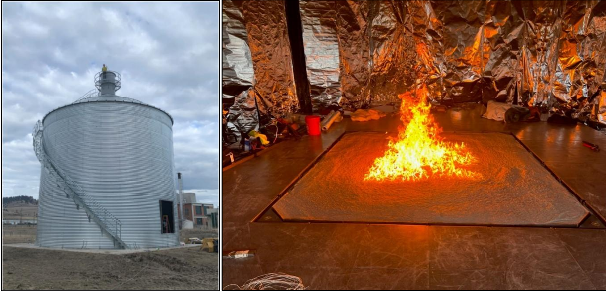
Photos showing the exterior (left) and interior (right) of the Grain Bin-Ventilation Controlled Combustion Facility at the U.S. Forest Service Missoula Fire Science Laboratory
